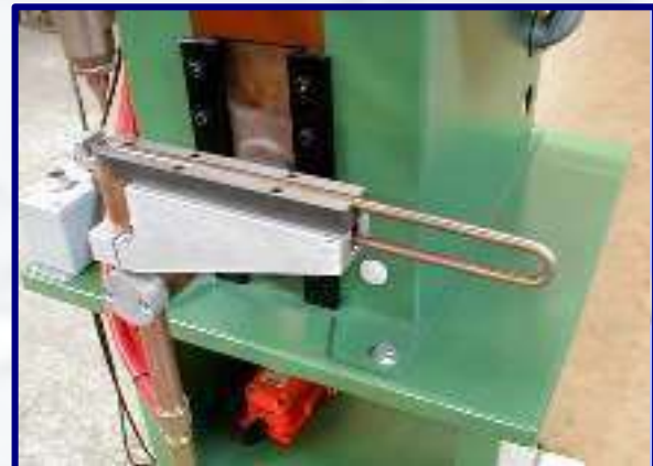
Element with 180 degree bend inserted into welding fixture
