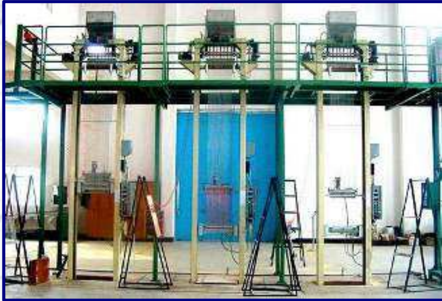
Three 24 Position Fast Fill Machines shown installed in a pit with a catwalk around the machines to facilitate loading MgO into the bulk hoppers and to provide access to the machine for changeover and maintenance. Also pictured are our pneumatic racks and our loading and unloading magazines.
