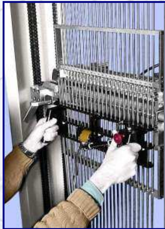
Pneumatic Rack Being Used to Insert 24 Tubes into Spring Clip Retainer Bar
