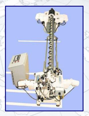
The Oakley Roll to Length Machine is designed to produce elements of a consistent length. The length of each element is precisely measured as it exits from the roll reducer, and then the elements are elongated in the Roll to Length Machine to the preset length.
