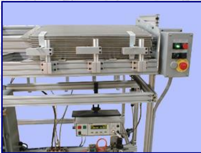
Feeder Controls and Hipot Test Unit
